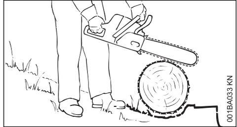
If on a slope, stand on the uphill side of the log. Watch out for rolling logs.
