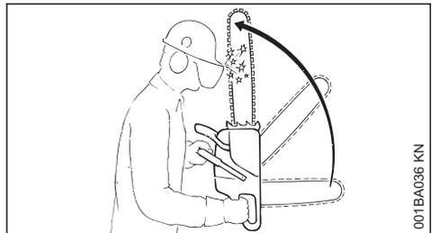
(Kickback) occurs when the saw is suddenly thrown up and back in an uncontrolled arc towards the operator.
