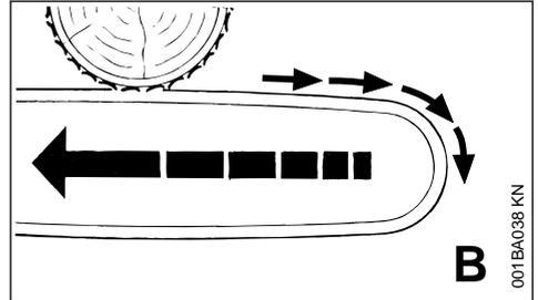
Pushback occurs when the chain on the top of the bar is suddenly pinched, caught or encounters a foreign object in the wood. The reaction of the chain drives the saw straight back toward the operator – **to avoid this risk:**
