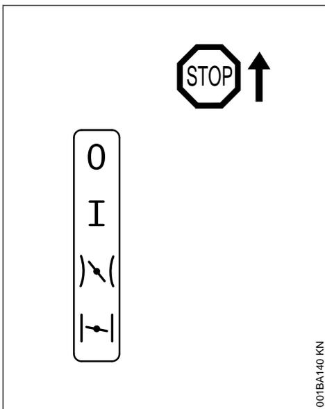
**Stop 0** – engine off – ignition is switched off
