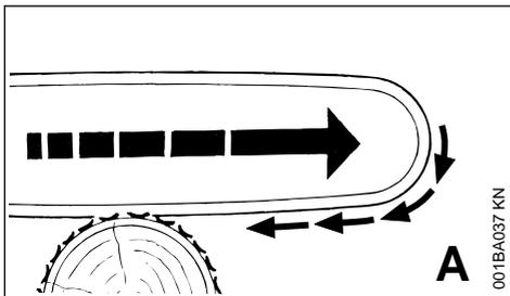
Pull-in occurs when the chain on the bottom of the bar is suddenly pinched, caught or encounters a foreign object in the wood. The reaction of
