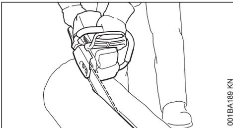
Sawing technique without use of the spiked bumper – risk of pull-in – position the guide bar as shallow an angle as possible – be especially careful – increased **risk of kickback!**
